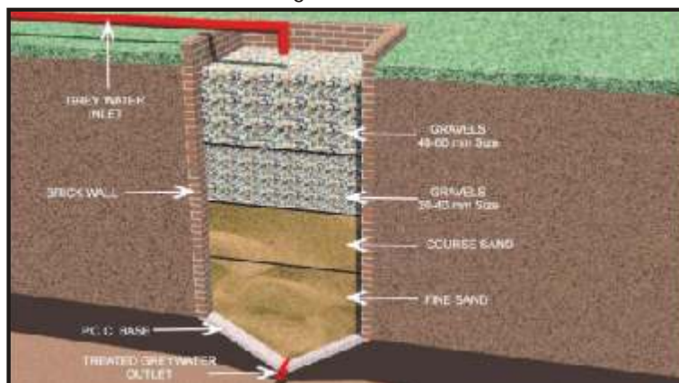
Figure 8 : Slow Sand Filter
