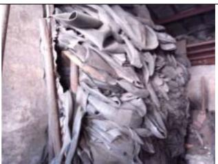
Tubes that are made 100% by raw natural rubber are exported to Pakistan, Sri Lanka, and Korea to be used for road construction. Tubes went through a recycling process usually is hard, and have less quality.
