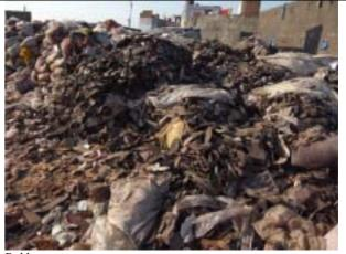
Rubber wastes. They are mostly shoe soles. At this point, shoe soles are taken off from shoes, which mean a preliminary sorting is occurring.
