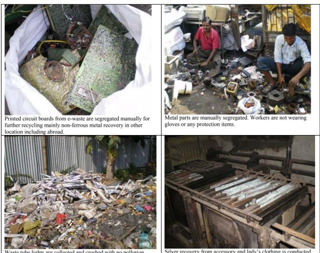
Waste tube lights are collected and crushed with no pollution control measures.
