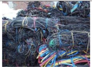
PVC cord in first stage recycling. (Rs. 28/kg) 1st stage PVC means it never recycled before. They are usually bendable, and more flexible.
